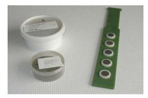
**Figure A.2.** Dried sample material in different containers ready for gamma measurements. To the right, <sup>99</sup>Tc preparations ready for counting.
