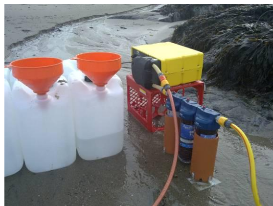
Figure 3.3. Filter system used for analysis of ^{137}\text{Cs} in sea water (Photo: NRPA).
