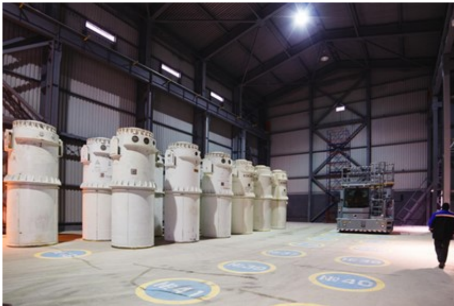
The spent nuclear fuel will be put in transport and storage containers that comply with international standards. (Photo: SevRAO).
