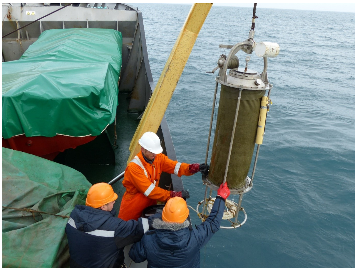
Figure 2.5. Collection of bottom seawater samples with CTD attached to water sampler (Photo NRPA).
