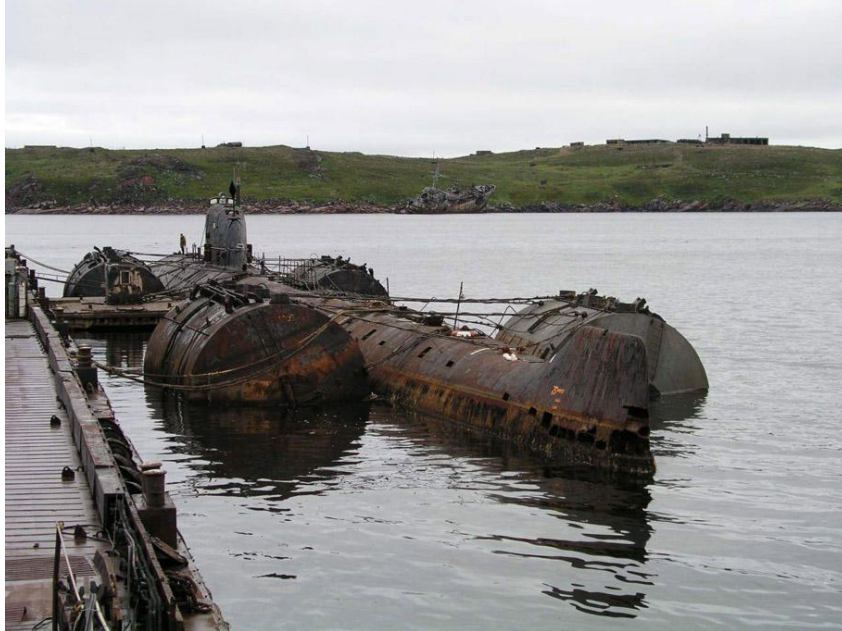
The nuclear submarine K-159 with the four floatation pontoons strapped to it prior to being towed. It sank during towing in August 2003. Photo: The Russian Northern Fleet.
