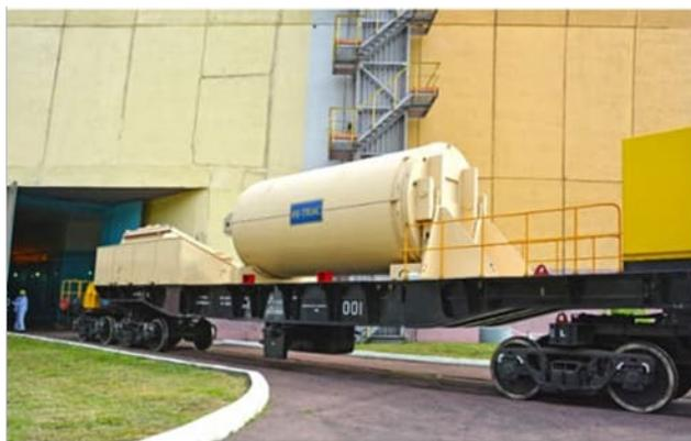
Fig. 3.2 –Holtec multipurpose canister and HI-TRAC cask
