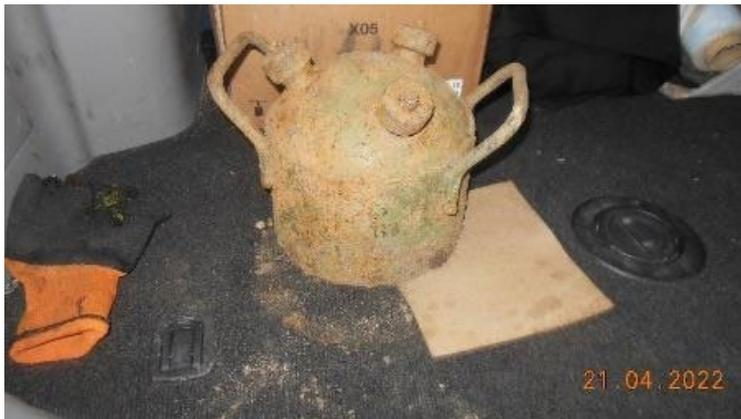
c) shielding unit with Cs-137 radiation source
