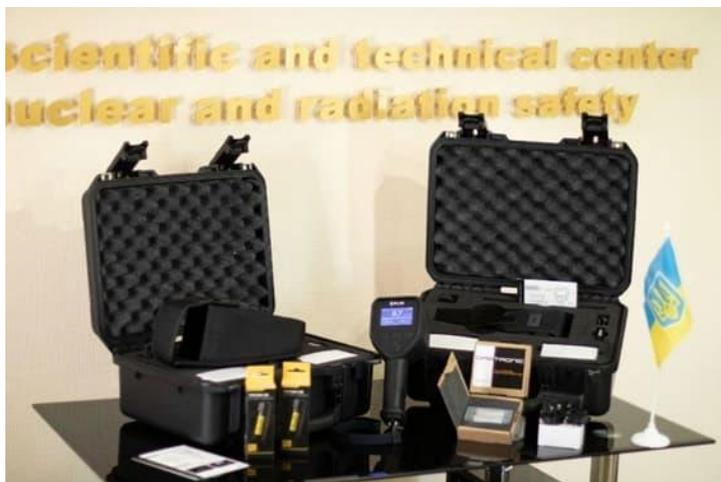
Figure 5.1 FLIR identiFINDER R425 gamma ray spectrometer
