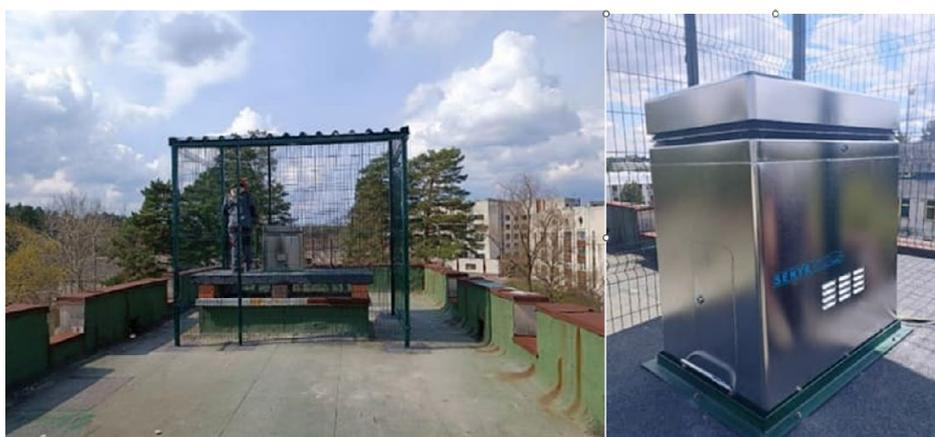
Figure 5.2 Radiation monitoring post based on the Goblin 200 air aerosol sampler located on the roof of the building of INTENSA Branch in Slavutych
