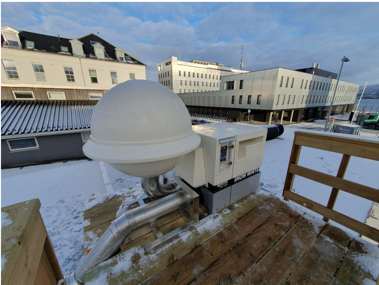
Figure 1. The high-volume air sampler at the Tromsø Fire and Rescue station (Photo DSA).
