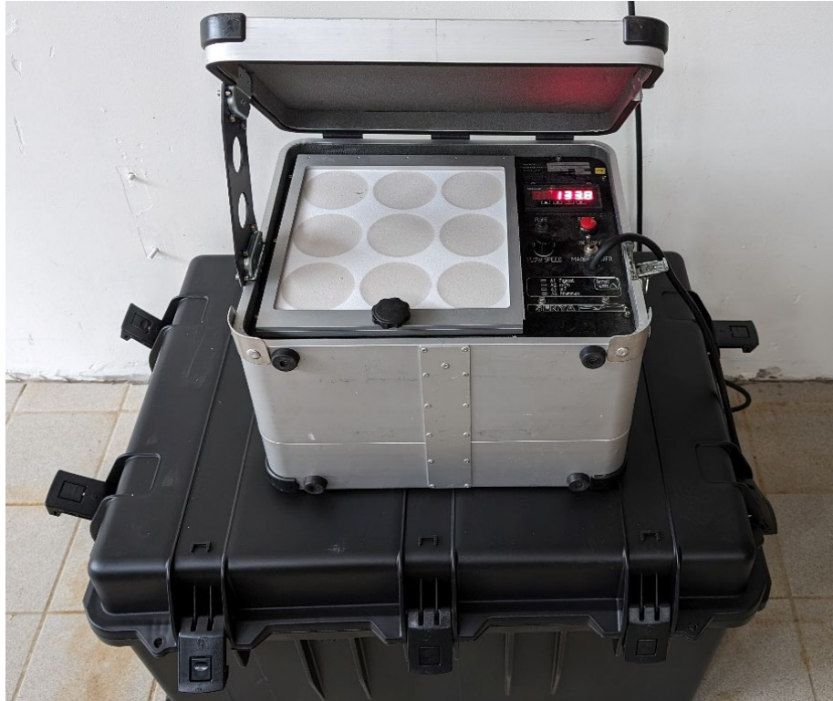
Figure 6. Close up of the Dwarf 100x9 portable air sampler at the end of a sampling period in the filtration room at the Breivika WTP showing particulate material trapped on the filter (Photo DSA).
