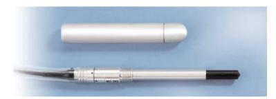
Figure 14: The ionization chamber type used in all measurements pictured along with its protective sleeve. The picture is taken from the product brochure. [31]
