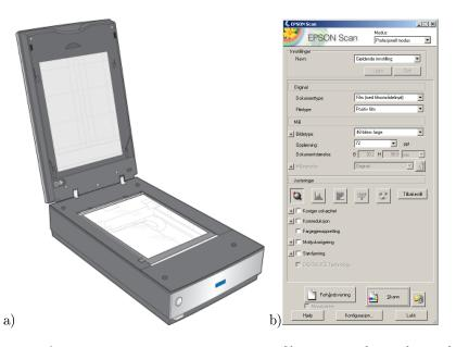
Figure 28: a) The Epson V750 scanner with the film area guide in place taken from the Epson Scan user's manual [49].b) Screen shot of the Epson Scan software with relevant settings.
