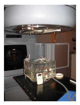
Figure 16: Ionization chamber setup for absolute dosimetry verification. The location of the ionization chamber is marked with a red circle. Picture taken at UUS.
