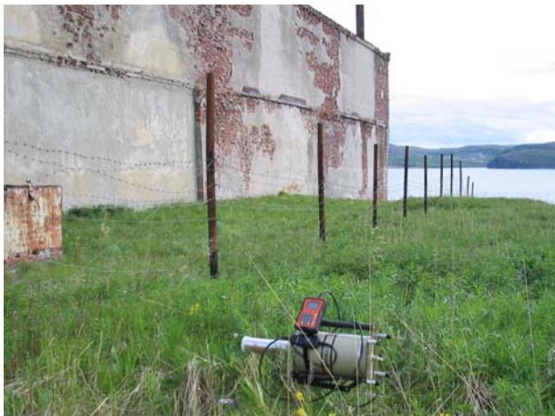
Measurements of gamma dose rate and measurements of radiation spectrum near building 5 on-site, SevRAO facility no. 1 at Andreeva Bay
