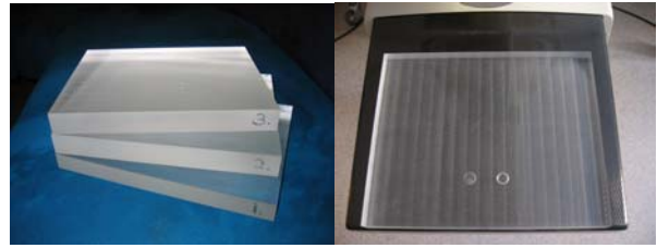
Test object consisting of PMM slabs.
