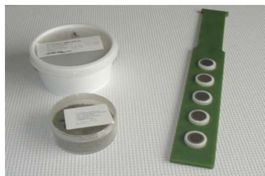
Figure A.2. Dried sample material in different containers ready for gamma measurements. To the right, ^{99}\text{Tc} preparations ready for counting.
