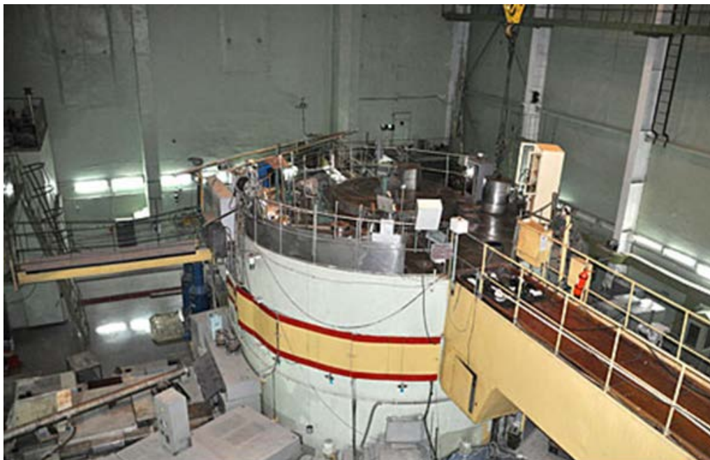
Figure 2.6 – Research nuclear reactor VVR-M of the Nuclear Research Institute of the National Academy of Sciences of Ukraine
