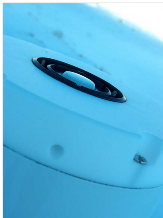
Figure 16. The front optics of the GUV multiband filter-radiometer. Photo: NRPA.
