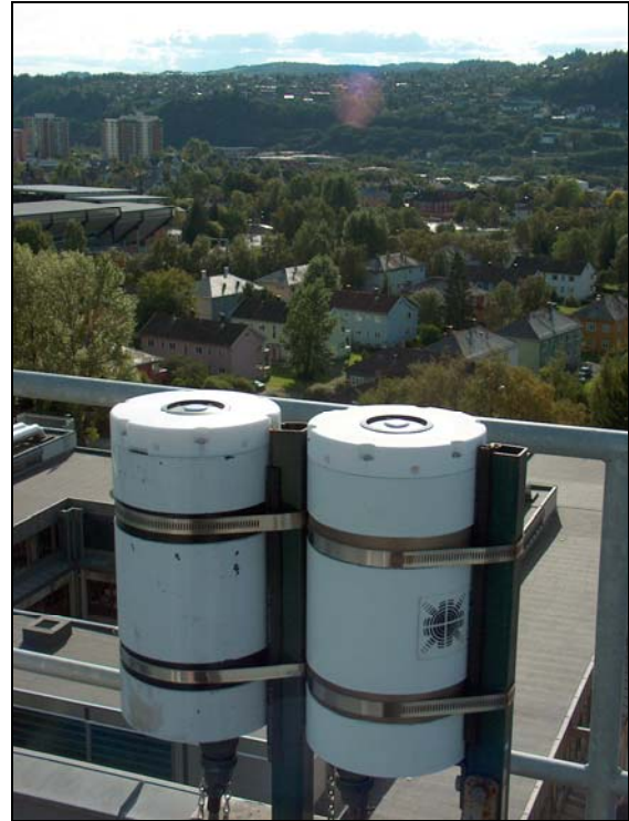
Figure 11. The GUV and the reference GUV in Trondheim. Photo: NRPA.
