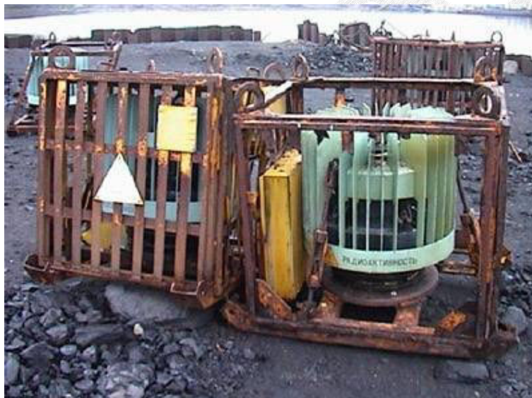
Retired RTGs awaiting decommissioning on the Kola Peninsula (Photo: Office of the County Governor of Finnmark).
