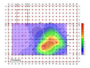
Fig. 5 The ADER field in Room 101 of Building 153 (top view) calculated by the Andreeva Planner Dose Calculator. (source: SRC-FMBC)
