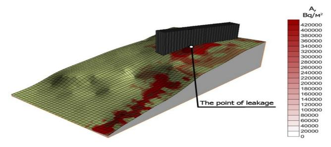
Fig. 1 Three-dimensional model of the distribution of surface activity in the area of the stream flowing out from under Building No. 5, Andreeva Bay STS (source: SRC-FMBC).
