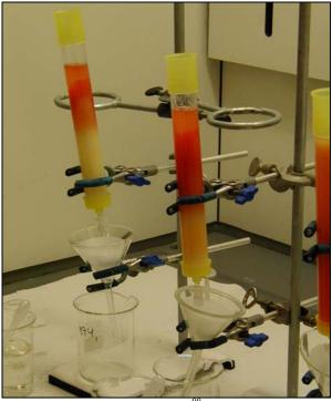
Ion-exchange separation of <sup>99</sup>Tc from sea water samples collected in the Norwegian Arctic.
