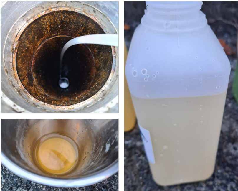
Figure 3 Image of well 1 (top left), the first drops of water pumped from the well (bottom left) and the sampled water after the well had been developed by pumping and surging until relatively clear water was obtained (right).
