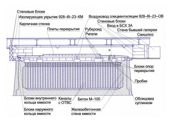
Figure 2. Vertical section through the DSU-3A tank along the diameter running north-south
