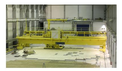
Figure 5. Handling machine above the DSU-2A tank.
