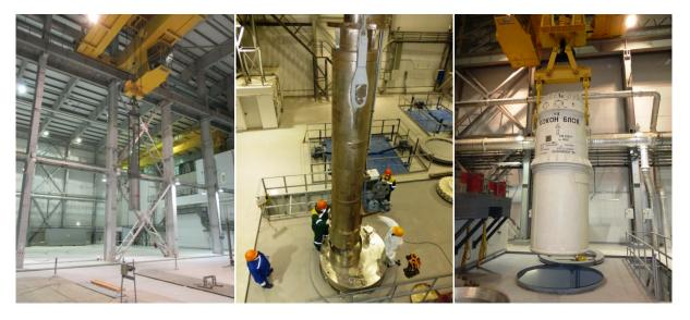
Figure 7. Process operations performed in the handling hall and TUK loading station in Building 153.
