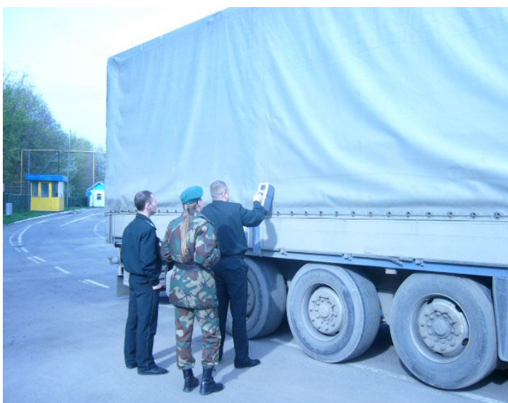
Fig. 4.7 – Inspection of vehicles with radioactive material at state border checkpoint
