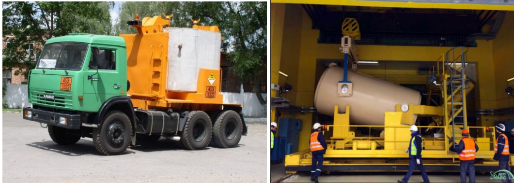
Fig. 4.5 – Vehicles for radioactive material transport
